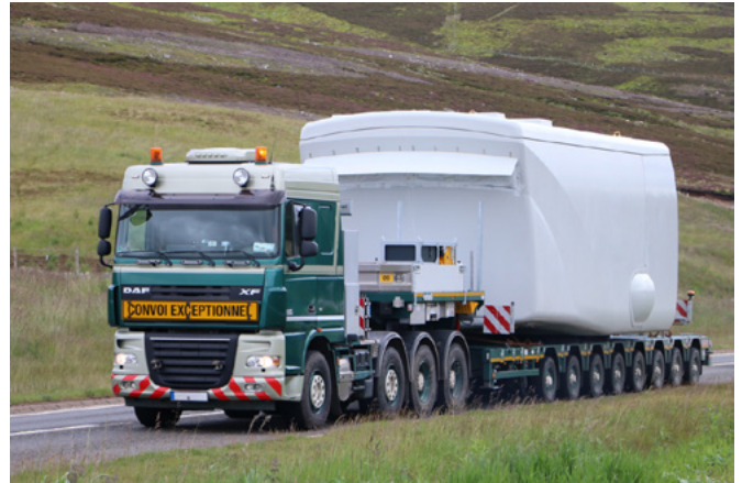
Figure 36: 4 axle tractor with 8 axle semi lowloader loaded with a nacelle
