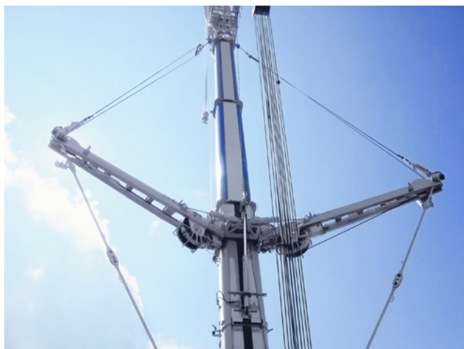
Figure 9: Rear view of a guying system on a telescopic crane
