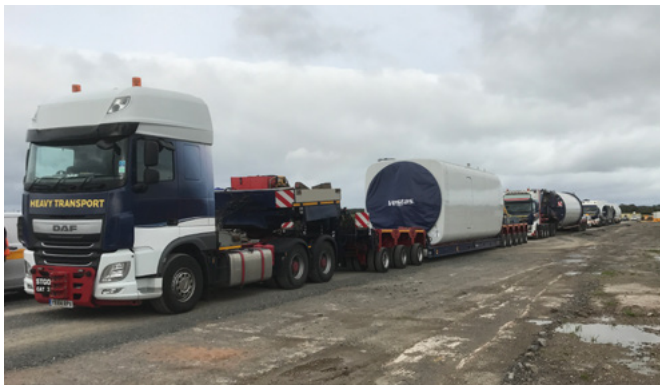
Figure 25: Typical wind turbine transport convoy
