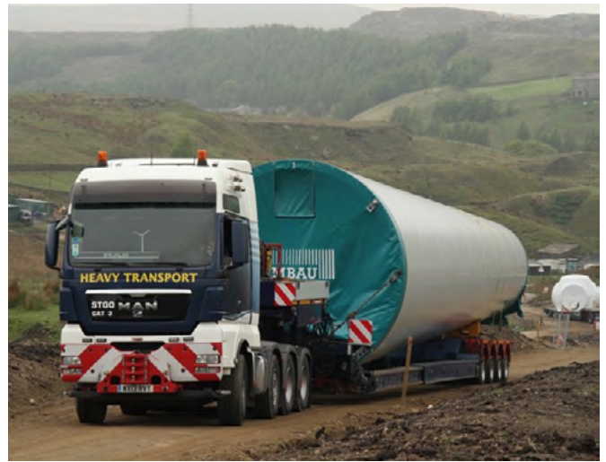
Figure 29: Typical WTG tower base section transport
