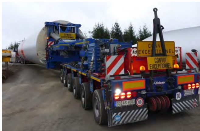
Figure 26: Tower transport using “clamps”
